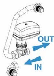
**Pompa scarico condensa**
